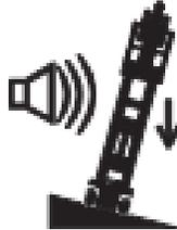
When the platform controls LED readout displays LL, the ground controls LCD displays LL: Machine Tilted, and the tilt alarm sounds at 180 beeps per minute, the following functions are affected: drive, steer, and elevate functions are disabled.
