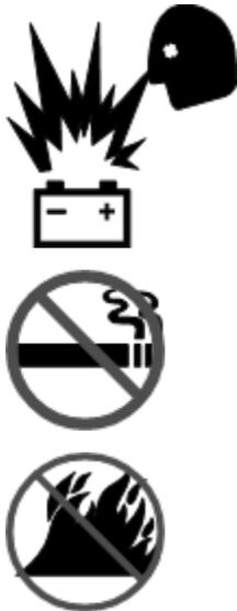
Keep sparks, flames, and lighted tobacco away from batteries. Batteries emit explosive gas.
