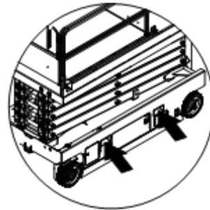
Position the forklift forks in position with the forklift pockets.
