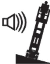
Return the machine to level ground to restore lift functions.
